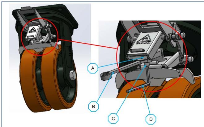
To adjust the distance between the brake and the wheel you need to:
